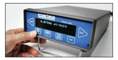
With that information from the calibration certificate, enter the full-scale mV/V using
