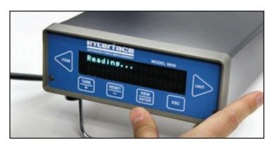
While the screen is displaying "Reading...", the 9840 is calibrating. Wait for just a few seconds for it to finish...
