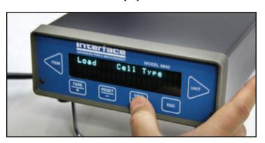
Select the measurement cell type that you are using. For this example, we are using a load cell, so we select "Load".
