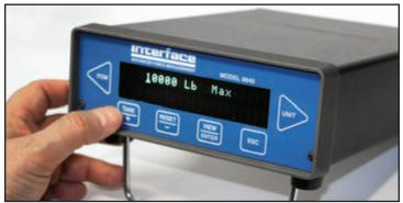
Next, you will need to refer to the sensor's Calibration Certificate. In it, identify the value for the max capacity and enter it into the 9840 using the same buttons: + , — , ◀ , and ▶.
