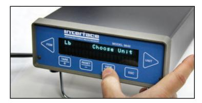
Select the necessary unit of measure and press **ENTER**.
