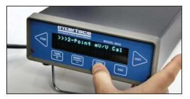
Using ▶, select ">>>2-Point mV/V Cal" and then press **ENTER**.
