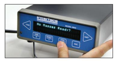
Check that there are no masses (no load) affecting the sensors so as to be sure that calibration begins with a zero balance.
