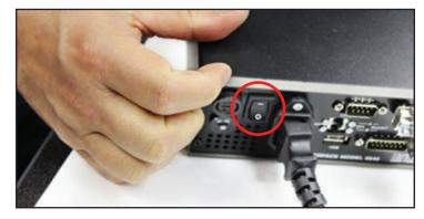
To turn on the 9840 Load Cell Connector, reach behind in the back corner and flip the switch up.
