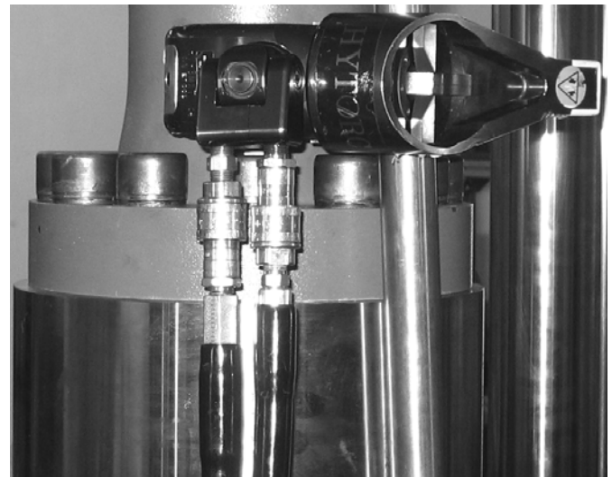
Using hydraulic Torque Wrench with reaction bar to tighten mounting screws on 2350.
